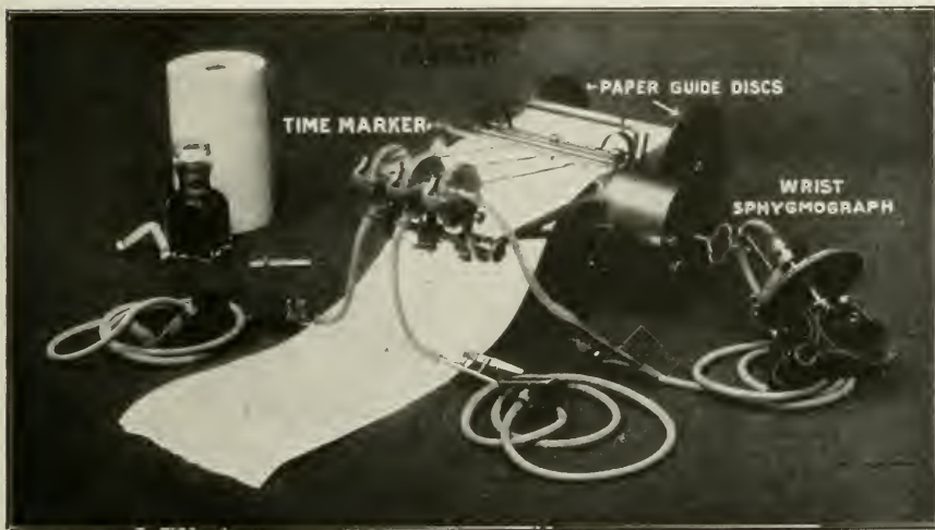
Fig. 2.—The Modified Mackenzie Ink Polygraph.
